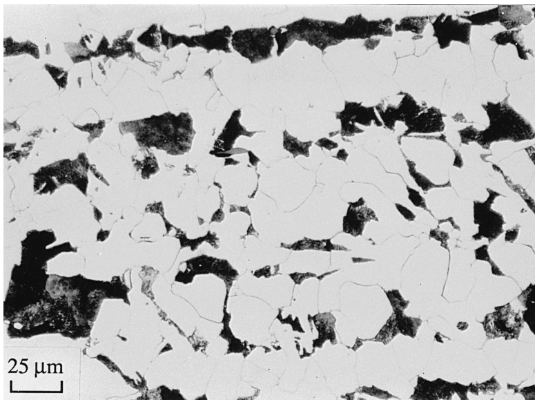
Fig. 1. Microstructure of normalized air cooled block 1 (reference).
