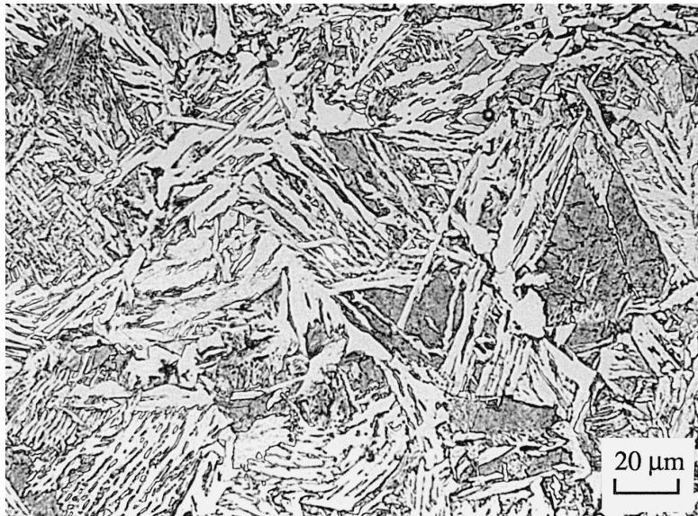
Fig. 3. Microstructure of austenized 1050°C water quenched block 3.
